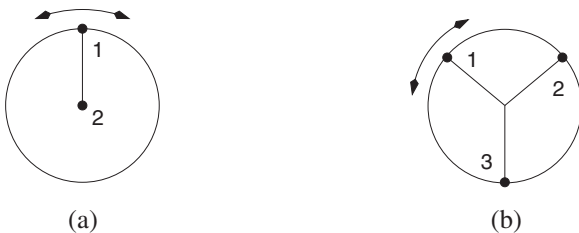
Fig. 3. Graphical interpretation of forces derived from potentials depending on two- and three-point distance functions. (a) Two particles interacting via a potential depending on two-point or pairwise distance. Holding particle 2 fixed and moving particle 1 on the circumference of the circle leaves the energy unchanged. This implies that the force on each particle is along the joining line, and that the resultant of the forces is zero due to the translational invariance of the energy. (b) Three particles interacting via a potential depending on three-point distance. Here any combination of the particles may be moved along the circumference of the circle without changing their interaction energy. This implies that for any distinct triplet the force on each particle is along a radial line from the center of the circle to the particle, and that the resultant of the forces is again zero due to the translational invariance of the energy.
